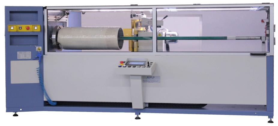
T/540 AUTOMATIC ROLL SLITTING MACHINE FOR FOAM, RUBBER AND FILMS
